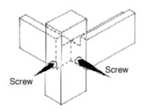
Ideally, the side supports should be attached at even intervals (every 30"), but you can modify this to suit your own requirements. Repeat for the other side, taking care to ensure that the routed groove points towards the middle of the shelving unit. Take the time to ensure that all joints are square; otherwise you may end up with a shelving unit that leans!
